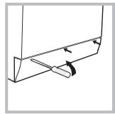
1. 以螺絲批鬆開機前部擋板(見圖); using a screwdriver, remove the cover panel on the lower front part of the washing machine (see figure);
